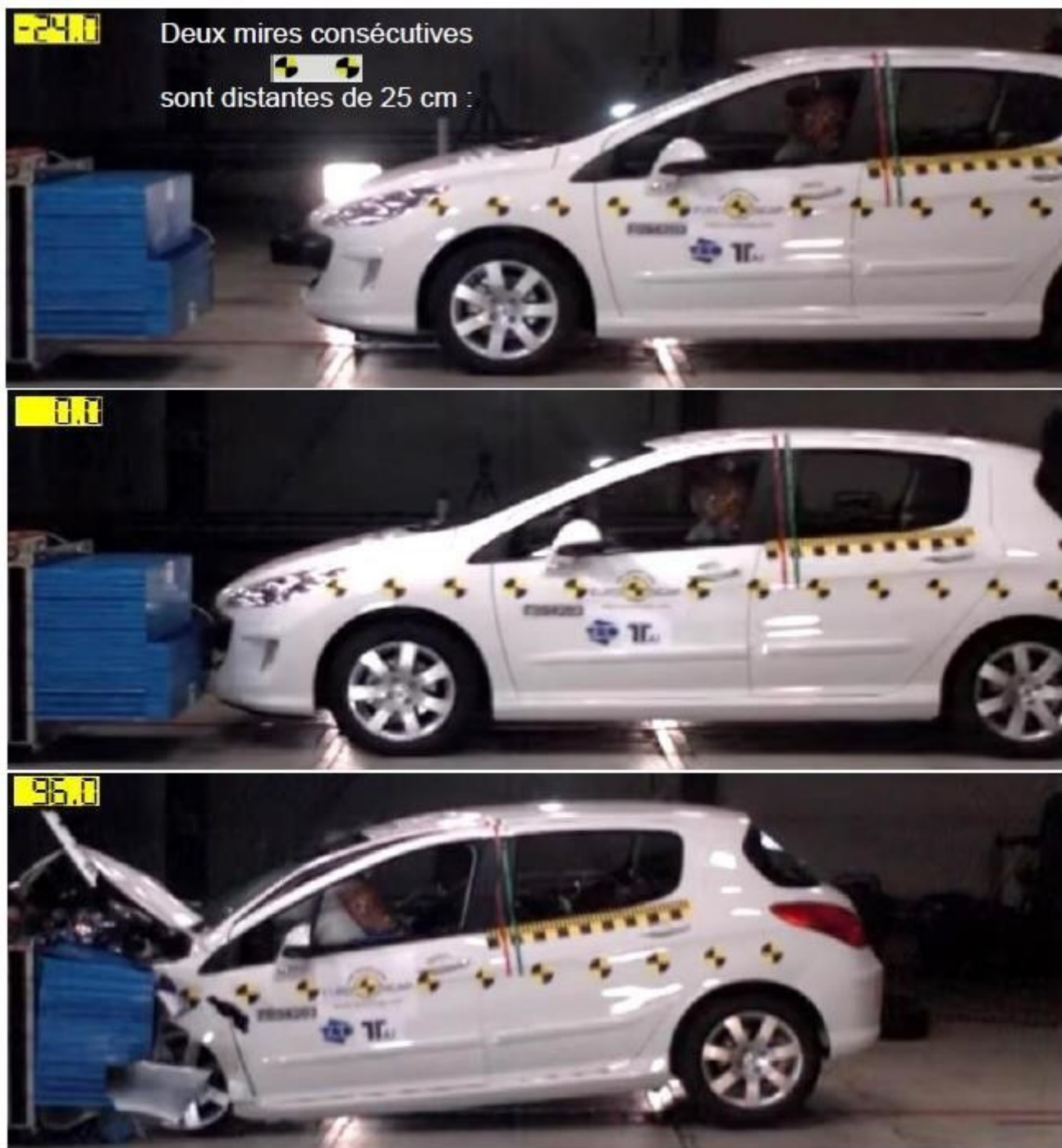
Figure 4. Photos du crash-test
